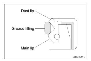
⑦ Fill the oil seal into the hole by using a oil seal guide and oil seal snap.
